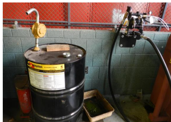
A designated barrel for used antifreeze that can be picked up by the offsite recycler (photo courtesy of Madison Park Vocational Technical High School)
