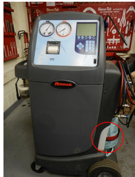
The front of a refrigerant recovery and recharging system (the circled refrigerant tank can be seen more completely above)
