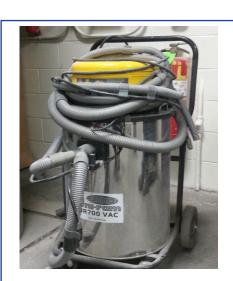
This portable vacuum sander has two adjustable arms that allow for two workers to sand simultaneously.
