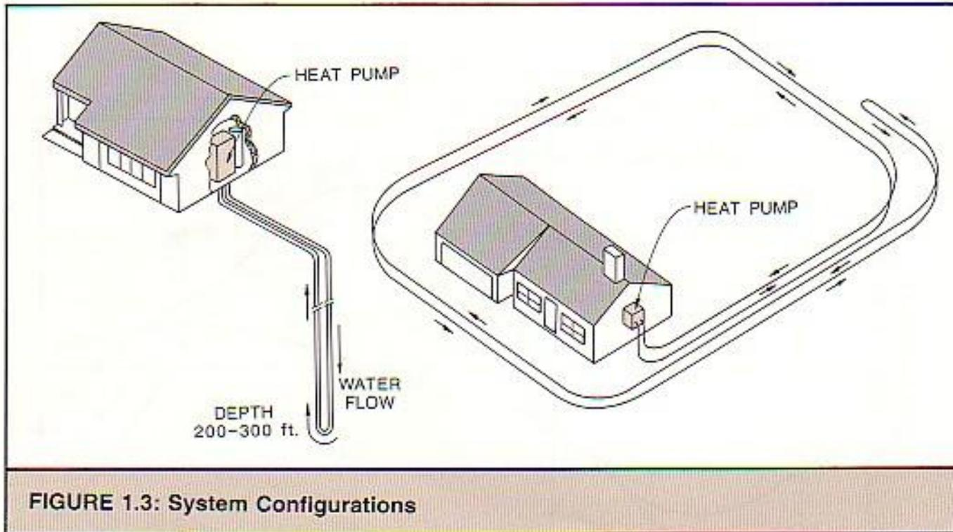
FIGURE 1.3: System Configurations
