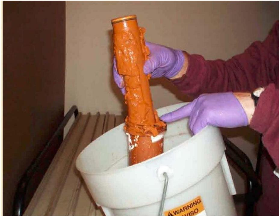
Iron sludge from a blocked strainer
