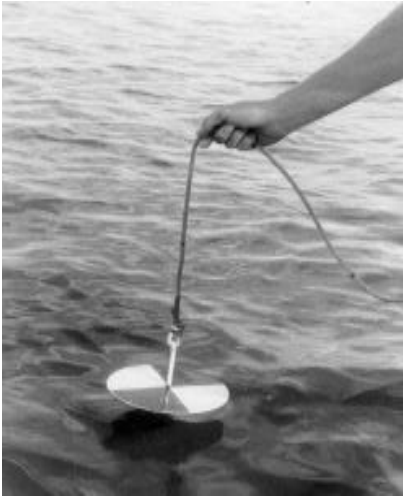
Figure 5. Secchi disk, an 8 inch disk painted in contrasting black and white pattern to determine level of light extinction.
