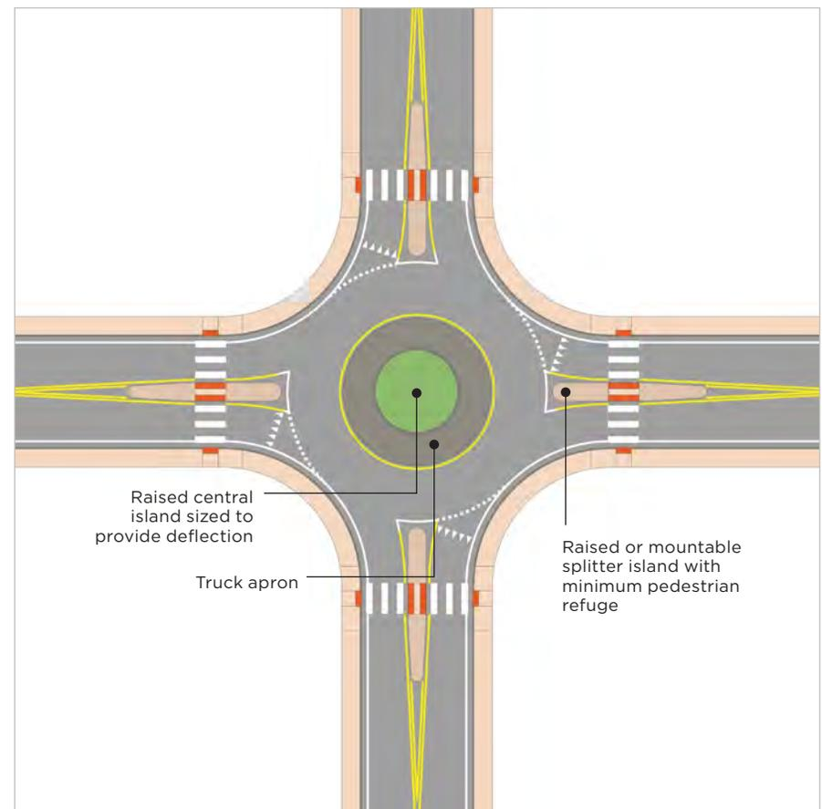
**FIGURE 5-30: MINI-ROUNDAABOUT CURBS OUTLINE WITH AN EXISTING INTERSECTION AREA IN STILLWATER, MN**
