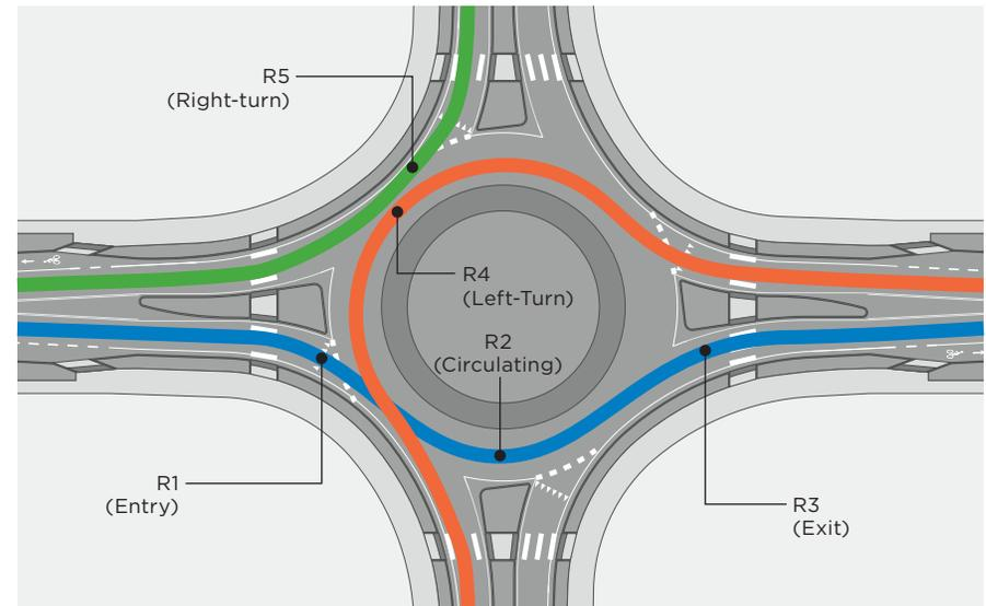
**FIGURE 5-11: FASTEST VEHICLE PATHS THROUGH A MULTILANE ROUNDABOUT**
