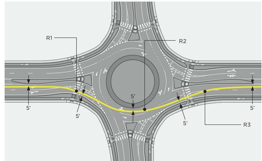
**FIGURE 5-12: FASTEST PATH DEVELOPMENT STEPS IN CAD**
