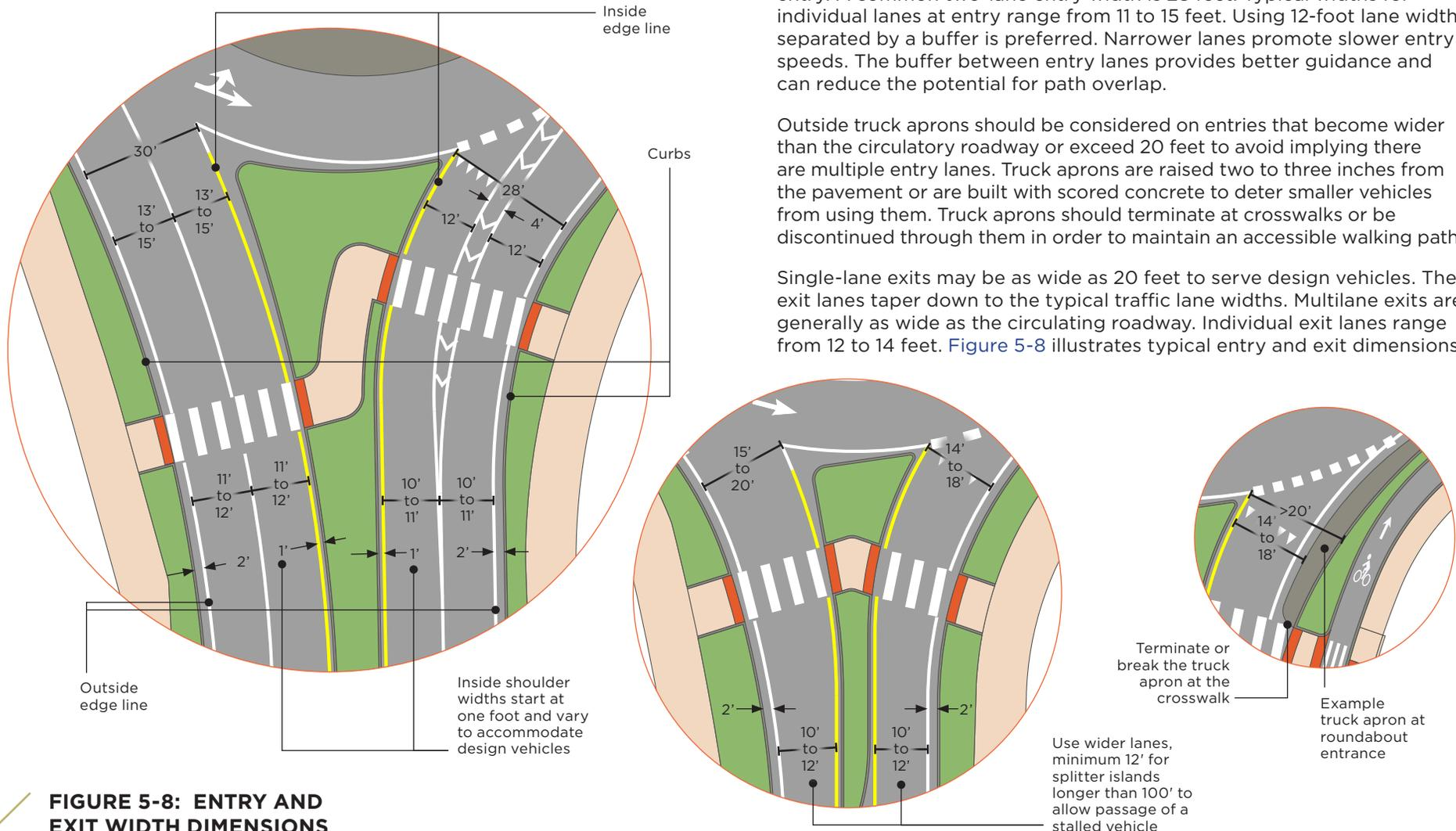
**FIGURE 5-8: ENTRY AND EXIT WIDTH DIMENSIONS**
