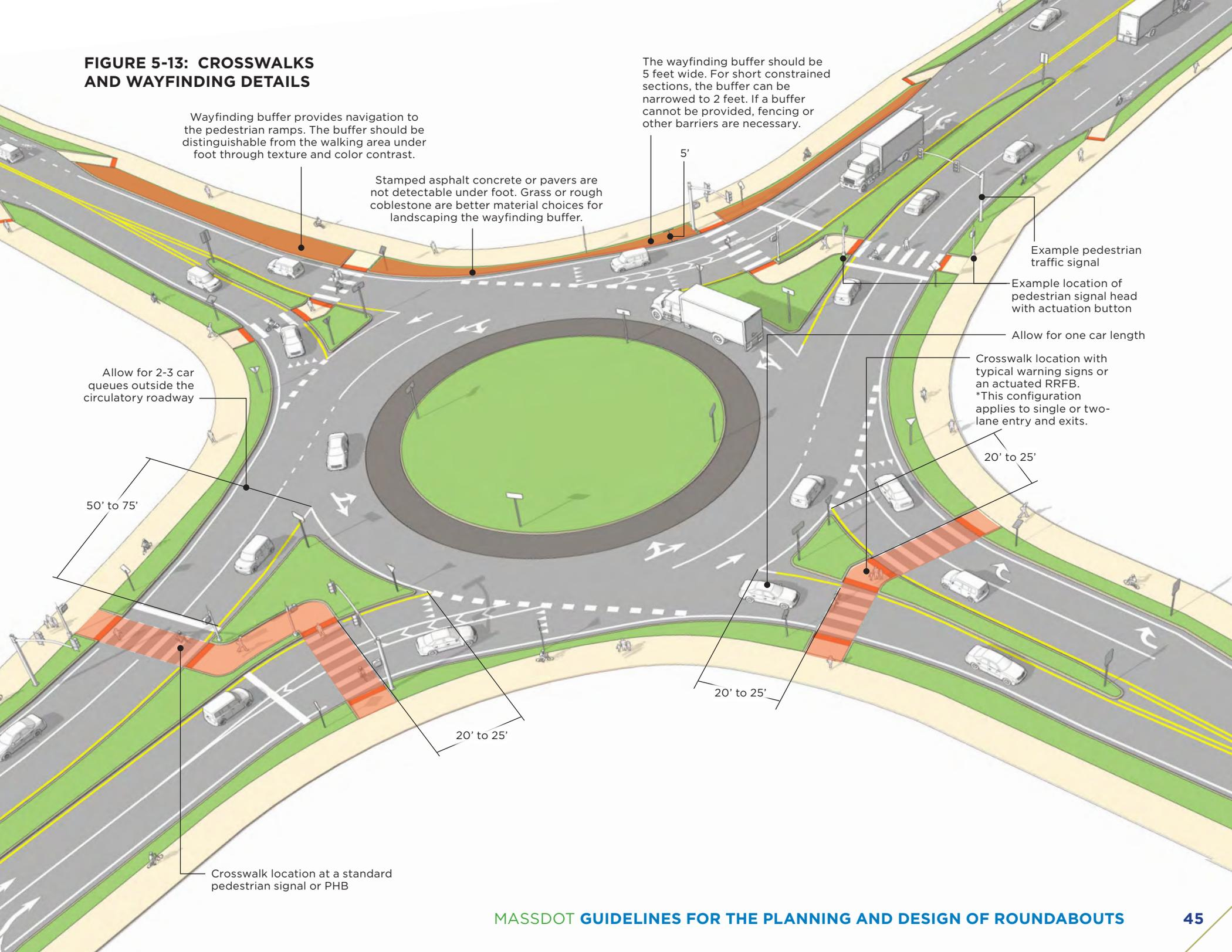
Wayfinding buffer provides navigation to the pedestrian ramps. The buffer should be distinguishable from the walking area under foot through texture and color contrast.
