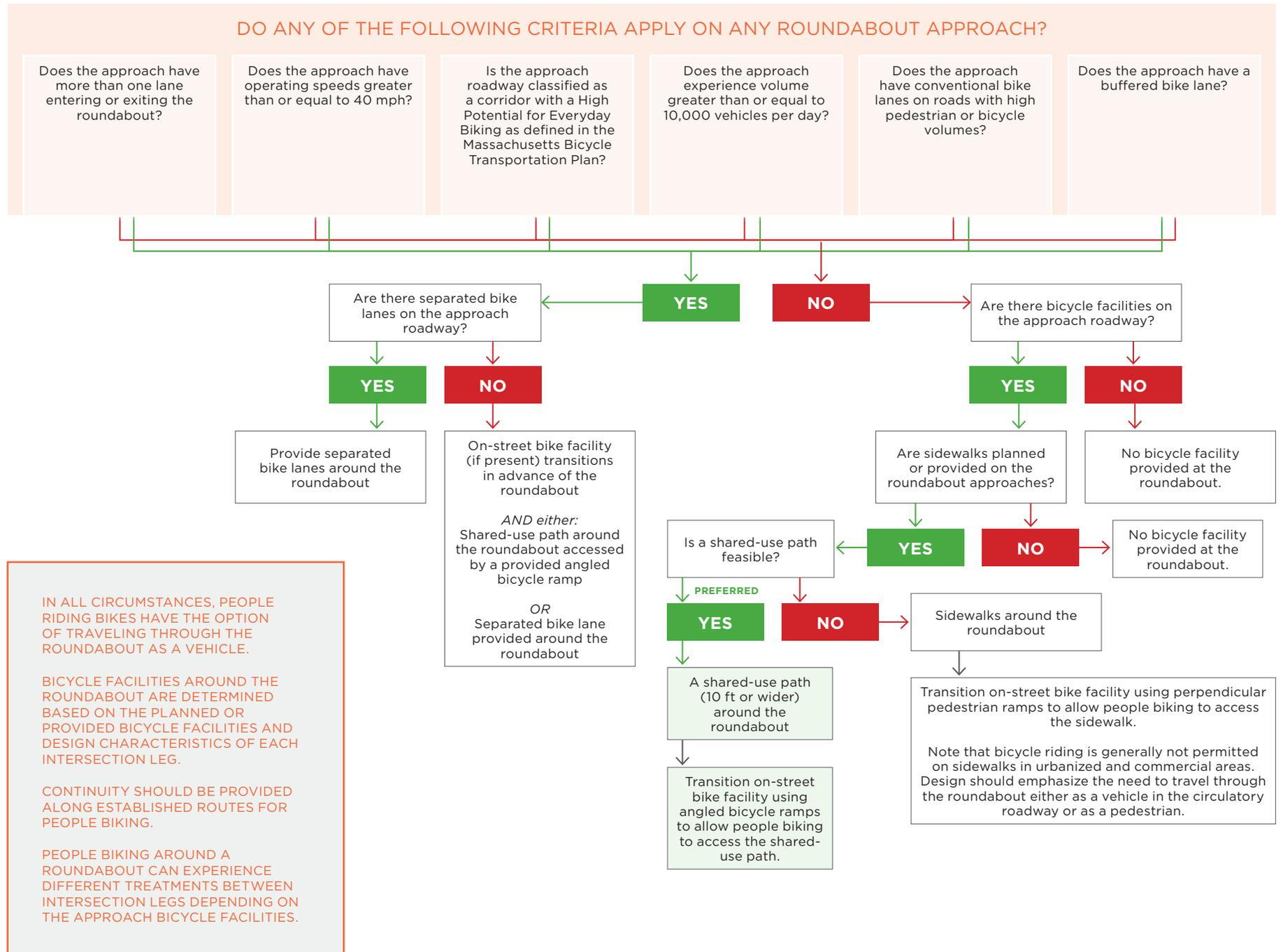
**FIGURE 5-18: BICYCLE MOVEMENTS AT A ROUNDABOUT**
