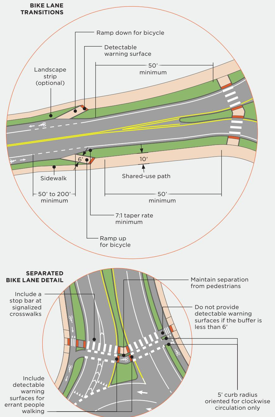
**FIGURE 5-17: BICYCLE FACILITY OPTIONS AT A ROUNDABOUT**
