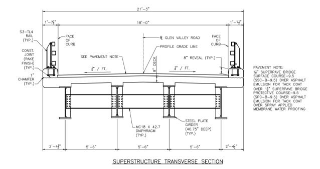
Approximately 400 feet of Glen Valley Road will be reconstructed. The road width within the project limits will be 18 feet wide. The proposed road width will transition to meet the existing width at the project limit. Existing guardrail within the project limits will be replaced with new steel highway guardrail. The profile will closely match the existing.
