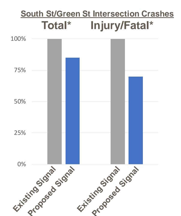
\*Based on Crash Modification Factors (CMF, which predict future crashes) for multiple types of geometric improvements. The use of CMF's are supported by Federal Highway and are widely used and accepted in the transportation industry.
