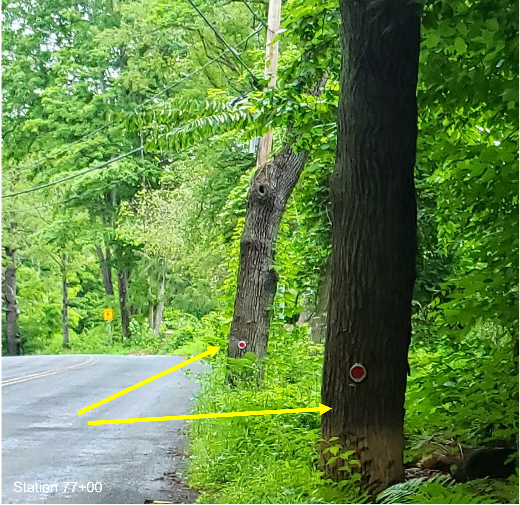
Close roadside objects in clear zone (trees, utility poles, rock ledge outcrops, steep slopes)
