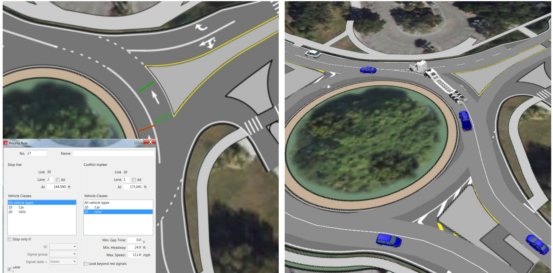
Figure 10: Using Priority Rules to Model No Passing of an Oversize Vehicle in a Multilane Roundabout
