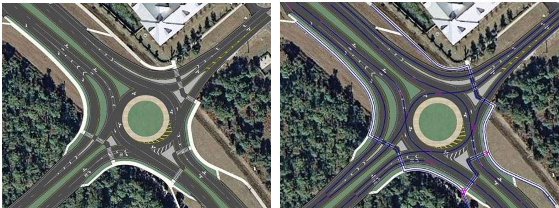
Figure 4: Modeling of Spiral Pavement Markings for Multilane Roundabouts in VISSIM
