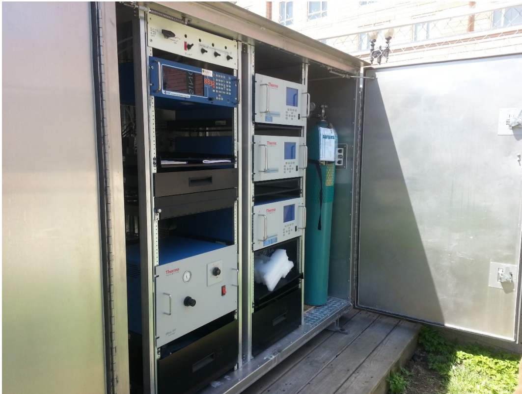
FIGURE 3-4: CO-NO-NO 2 DST MONITORS ENCLOSURE
