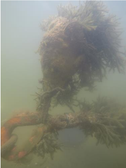
Figure 20. Subsurface buoy and rode of mooring 134 fouled with Codium
