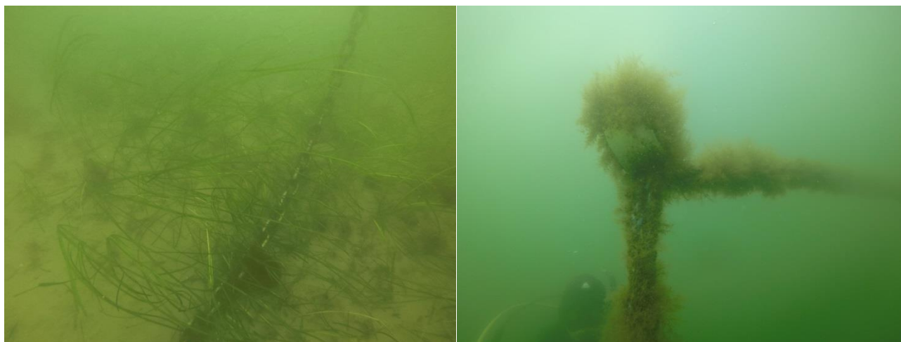
Figure 5. (left) Mooring 747 chain partially dragging through eelgrass; Figure 6. (right) Mooring 717 subsurface buoy floating gear and functioning properly
