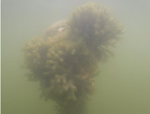
Figure 26. Heavily fouled subsurface buoy at mooring 1307/525
