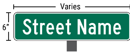
Figure 18. Size street name signs for shared use paths at 6 inches in height
