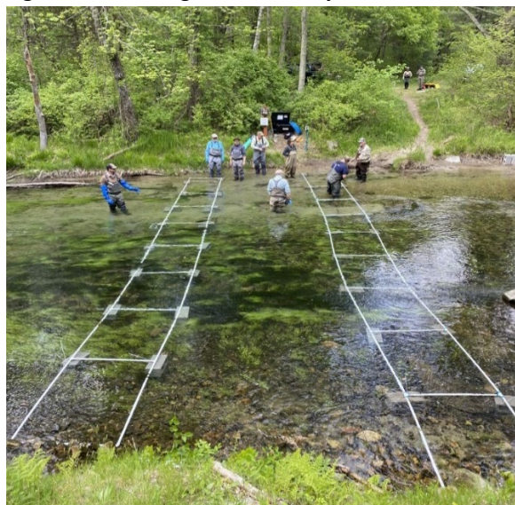
Figure F 12. PIT tag antenna array in the Swift River
