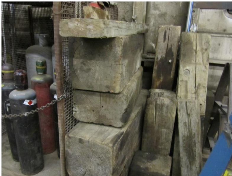
Figure 3 – The oak block cribbing being used during the incident
