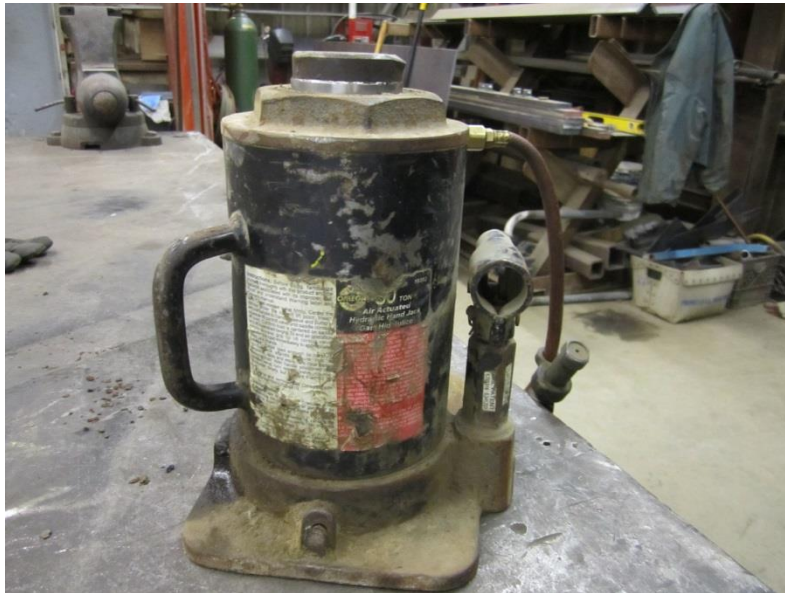
Figure 2 – The 30-ton bottle jack being used during the incident
