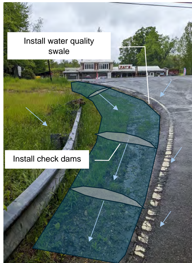
Photo 8-2: Erosion along the shoulder of the road
