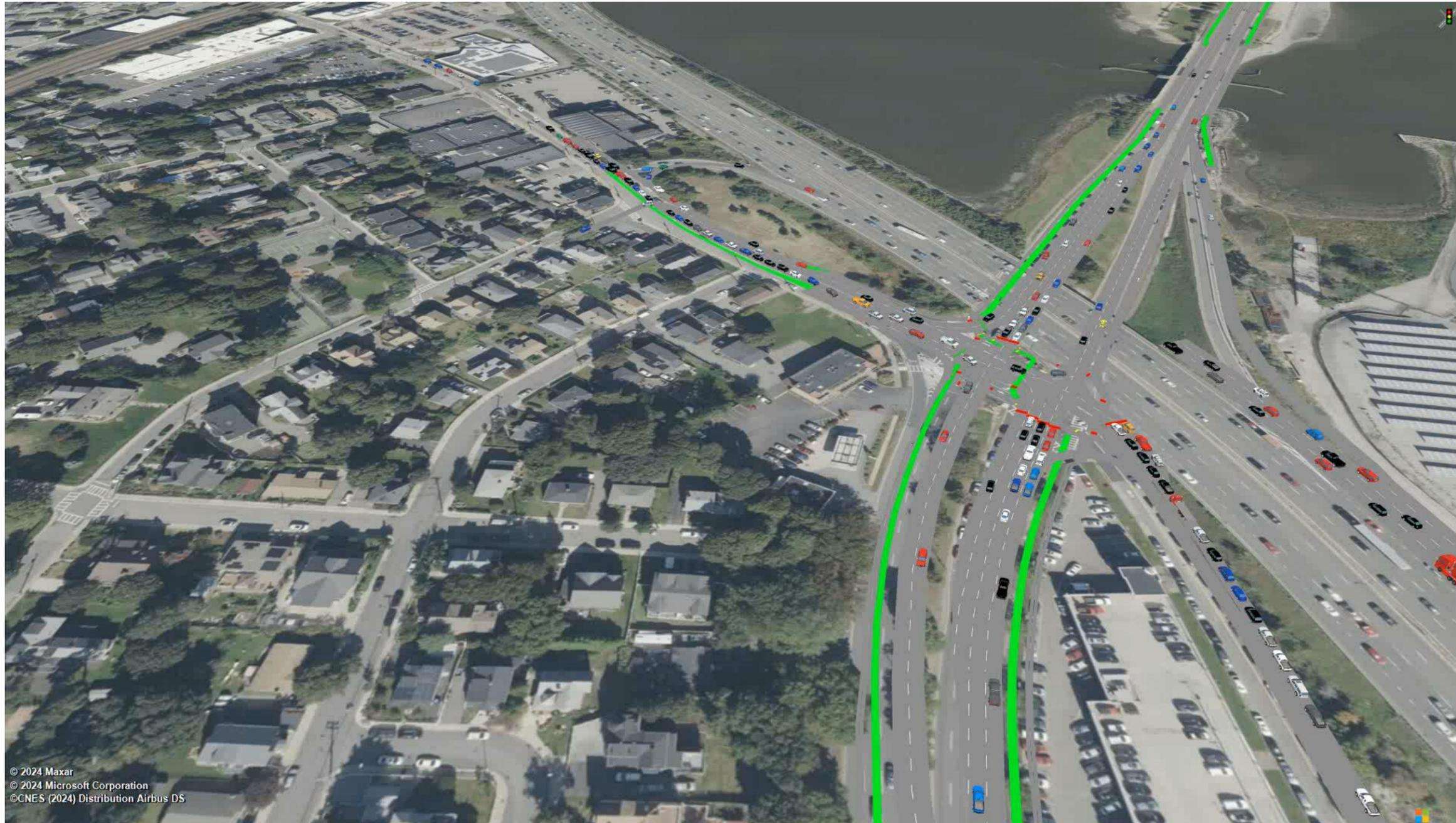
The model simulates multimodal movements through Freeport Street for the Modified DCR Design option
