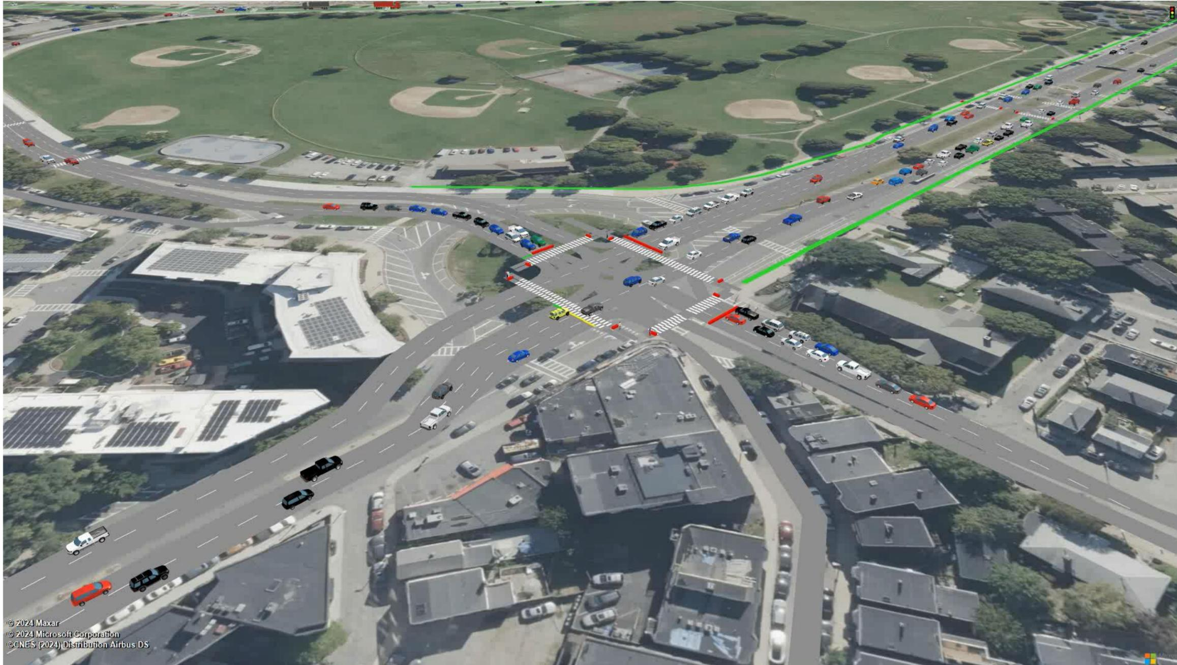
The model simulates multimodal movements through Preble Circle for the Signalized Control option
