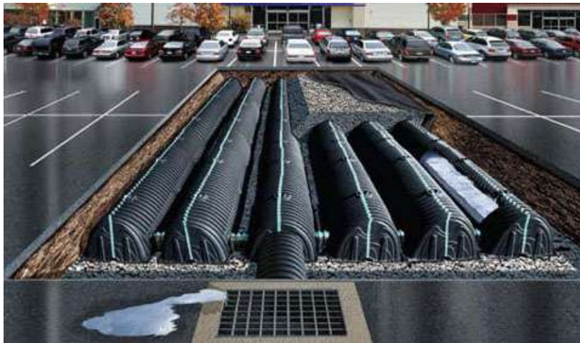
Cutaway View of Temporary Underground Stormwater Storage
