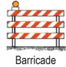
In addition to posting orange warning signs, road work crews can use a number of channeling devices to keep traffic in lanes and away from hazards. Sometimes, electric warning arrow signs will direct traffic flow near a work zone.
