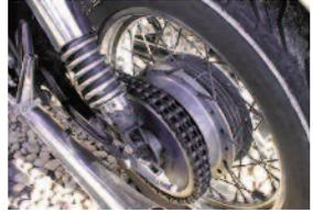
A rider will recognize a chain break due to the instant loss of power to the cycle's rear wheel. If this situation should arise, roll off and close the throttle while gently braking to a safe stop at the road's edge. Chain slippage or breakage can be avoided through routine and proper maintenance.
