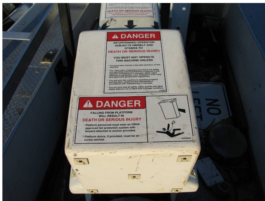
Figure 2 – Vehicle-mounted aerial lift fall hazard danger decal
