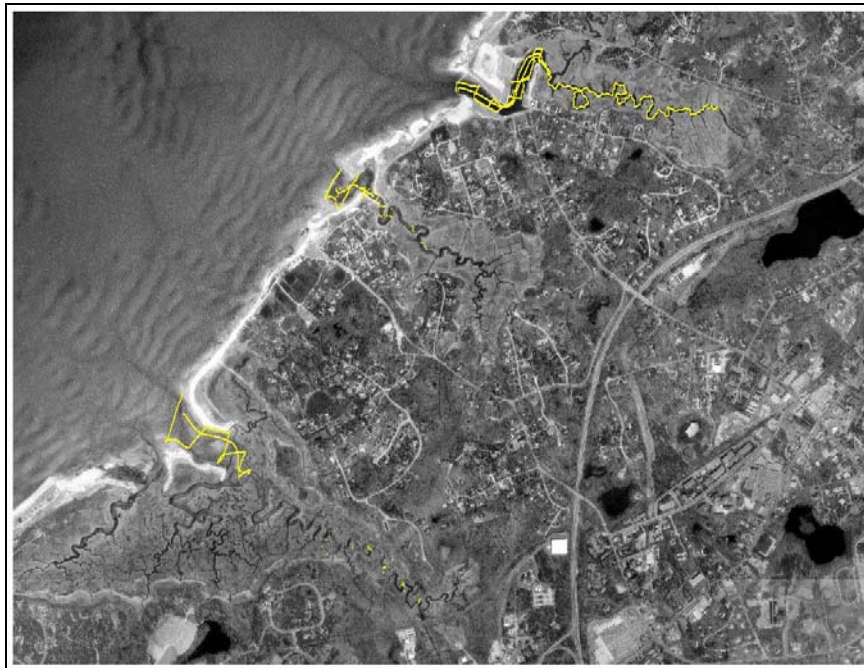
Figure V-2. Actual paths followed by recent (Fall, 2001) survey boat during bathymetry surveys of the Cape Cod Bay embayments of Orleans, MA. Fathometer paths are plotted on a composite 1994 aerial photograph of the area.
