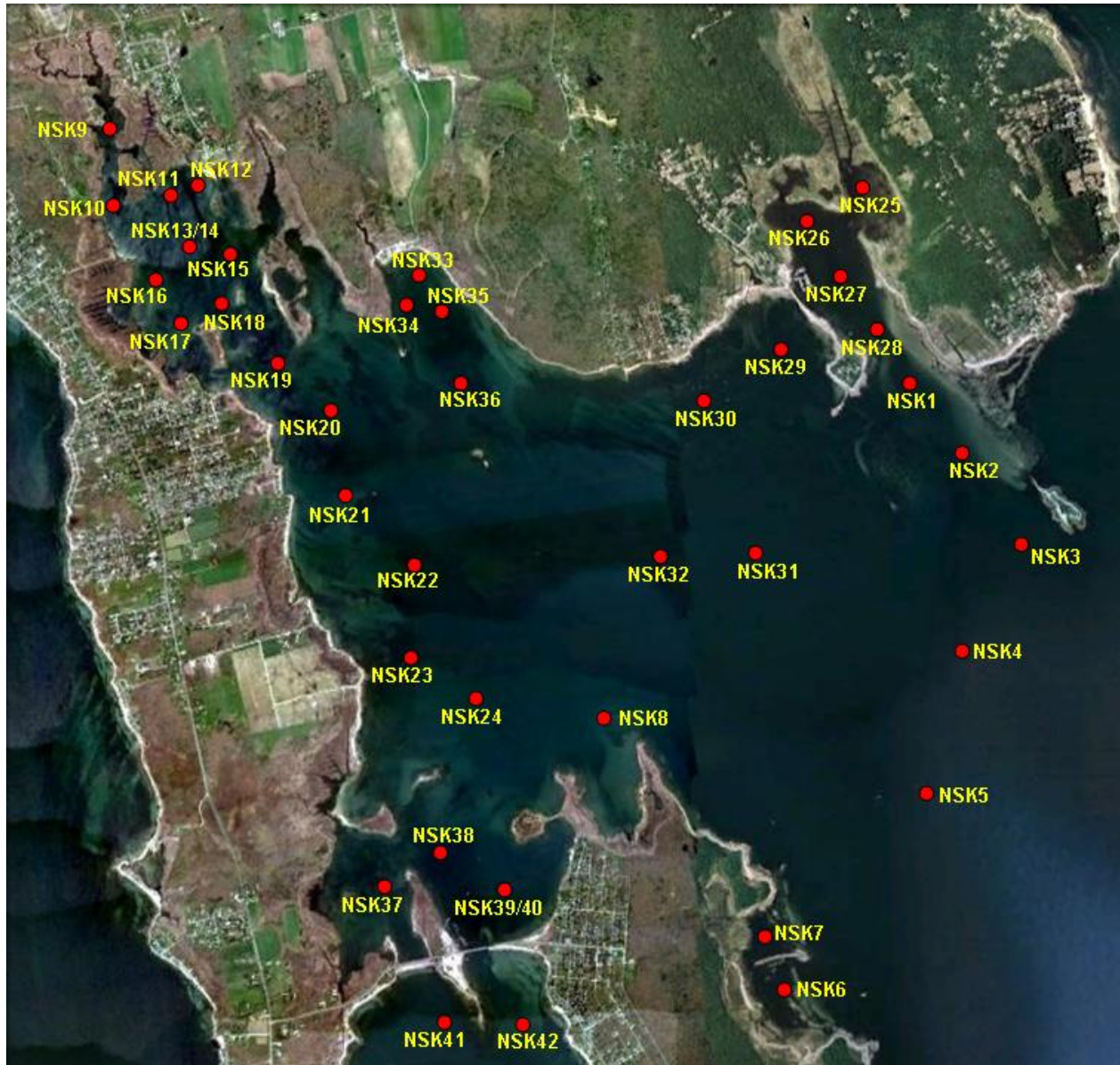
Figure IV-11. Nasketucket Bay / Little Bay Estuary sediment sampling sites (red symbols) for determination of summer nitrogen regeneration rates. Numbers relate to the reference list of cores presented above.
