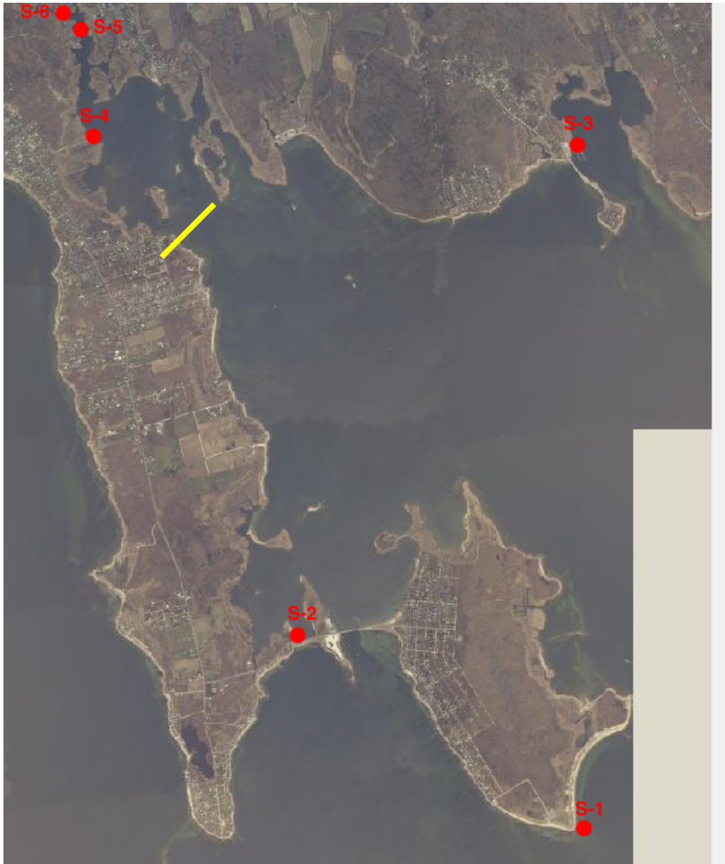
Figure V-2. Aerial photograph of the study region identifying locations of the tide gauges used to measure water level variations throughout the system. The six (6) gauges were deployed for at least a 37 day period between March 28, and May 24, 2006. The red dots represent the approximate locations of the tide gauges: (S-1) represents the gauge in Buzzards bay (Offshore), (S-2) east of West Island, (S-3) inside Brandt Island Cove, (S-4) inside Little Bay, (S-5) north of Little Bay in the marsh, and (S-6) north of Little Bay near the culvert on Pierces Point. The ADCP transect line is shown in yellow.
