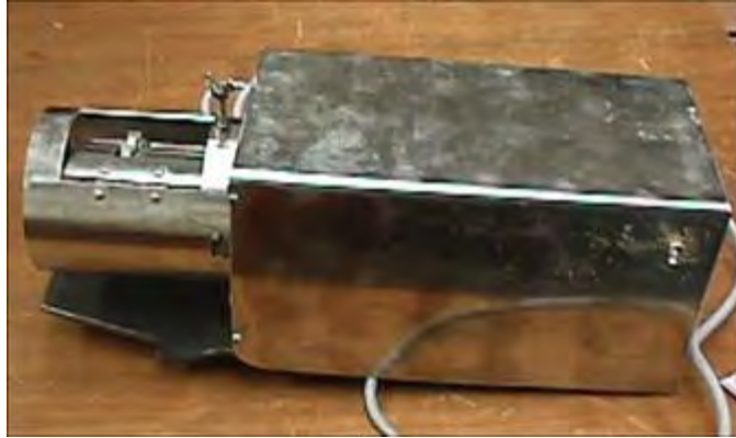
Figure 23 – Mechanical stainless steel oyster grinder
