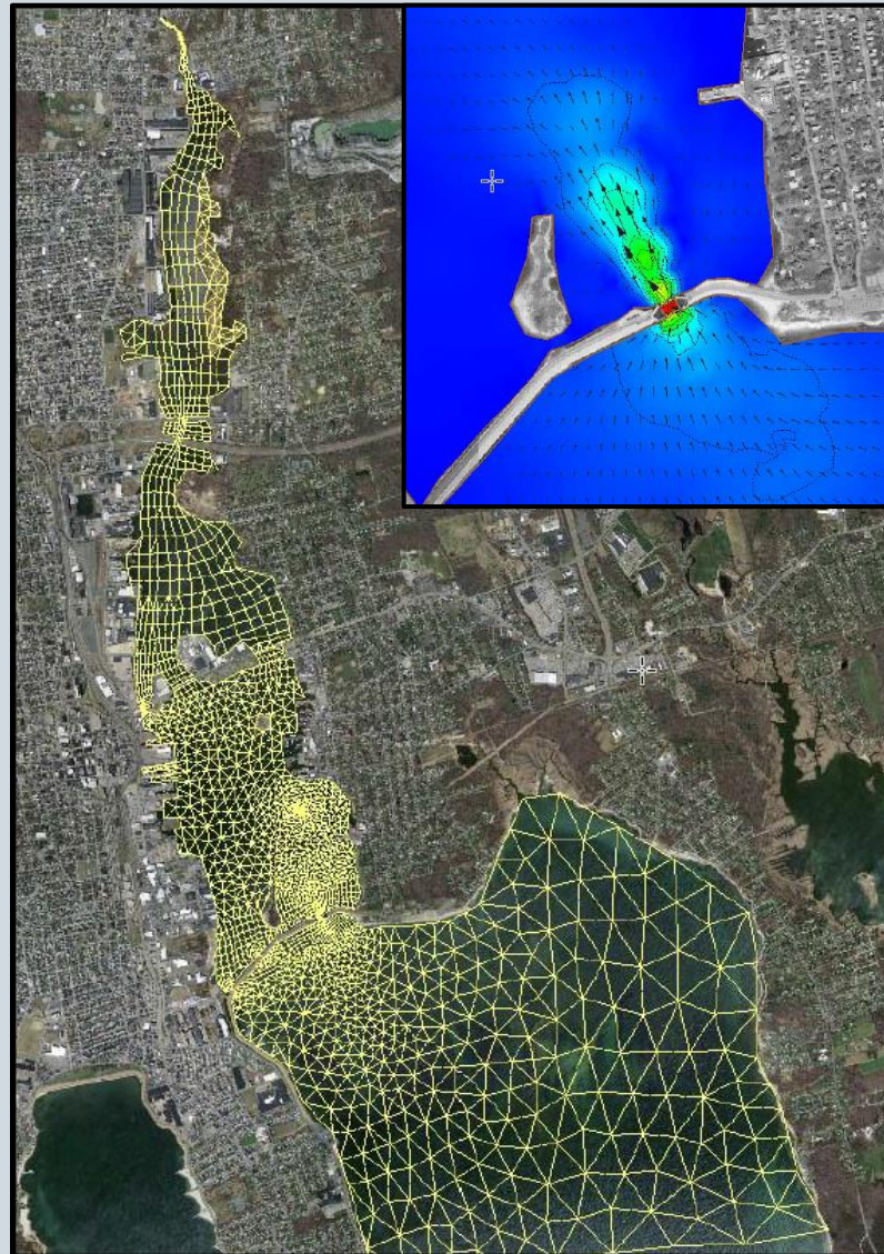
Hydrodynamic Model Grid Mesh & Example Model Output
