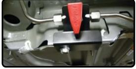
1/4 Turn Shut-Off Valve, Off Points Down
