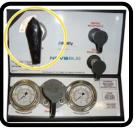
Emergency Shut-Off Valve (OFF position)
