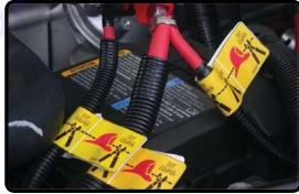
**Cut 3 Exposed Cables (Alternate Procedure)**
