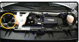
**Disconnect the 12V Battery Cables**
