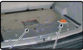
HV Battery Pack HV Service Disconnect Switch
