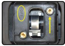
**HV System Disconnect Switch**
