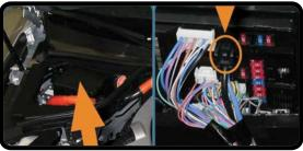
**Fuse and Box in Engine Compartment**
