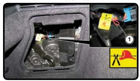
**Alternate HV Disconnect Cutting Solution**
