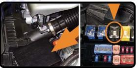
**Fuse and Box in Engine Compartment**
