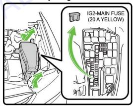
Remove Fuse IG2 in Engine Compartment
