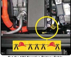
Cut the 12V Negative Battery Cable and DC to DC Converter Cable
