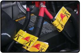
**Cut 3 Exposed Cables (Alternate Procedure)**
