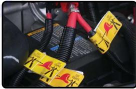
Cut 3 Exposed Cables (Alternate Procedure)
