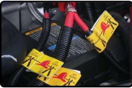
**Cut 3 Exposed Cables (Alternate Procedure)**
