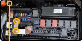
**Cut Cable and Main Fuse Screw Locations**
