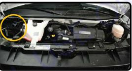
**Disconnect the 12V Battery Cables**
