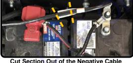
Cut Section Out of the Negative Cable
