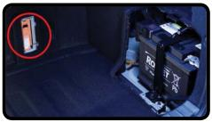
12V Battery and Service Plug in Trunk
