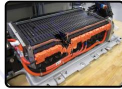
**Damaged High Voltage Battery**
