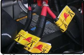
**Cut 3 Exposed Cables (Alternate Procedure)**
