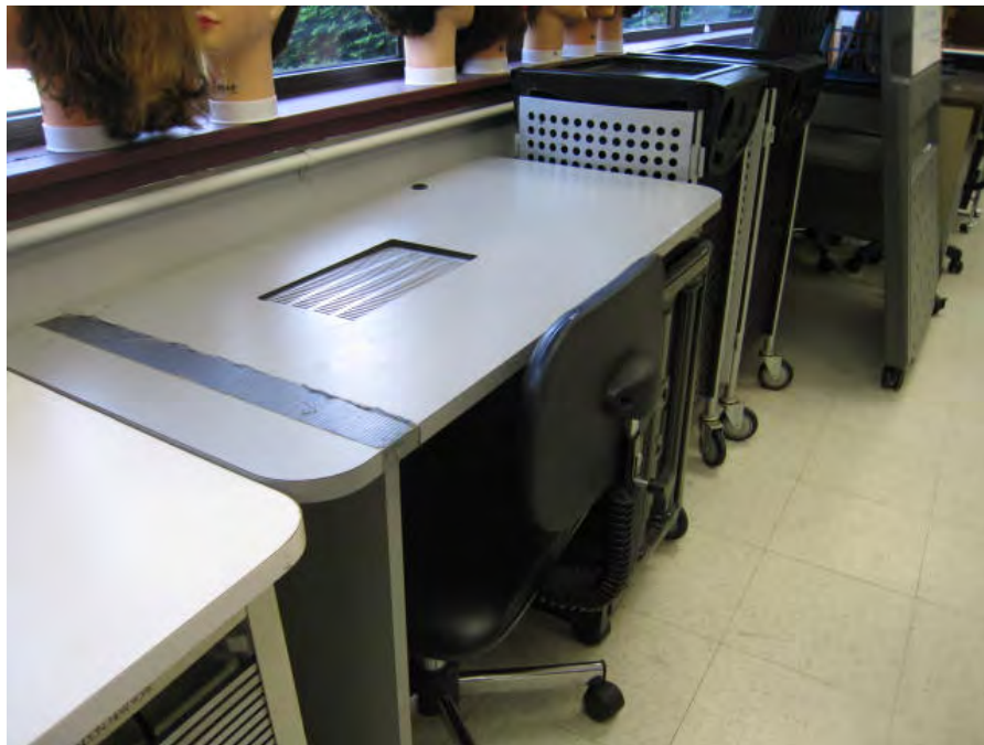
Mechanically-vented manicure table
