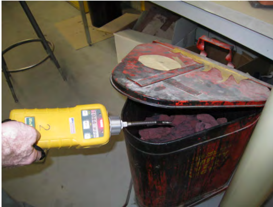
Oily rag storage container; unit was tightly sealed so VOCs could only be detected with the lid open
