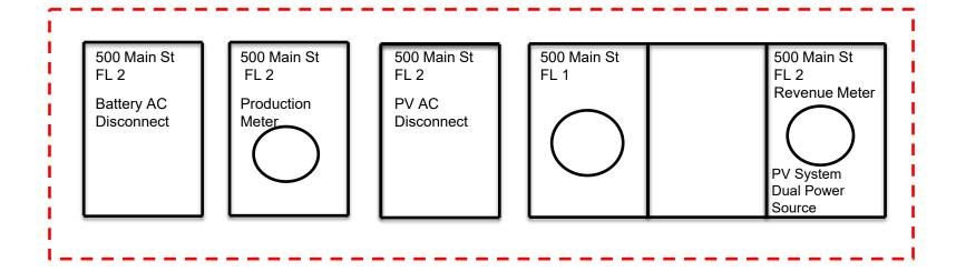
Note: All the Revenue Meters, Disconnects and Production Meters are grouped together on the exterior either on the front, or sides of the buildings.
