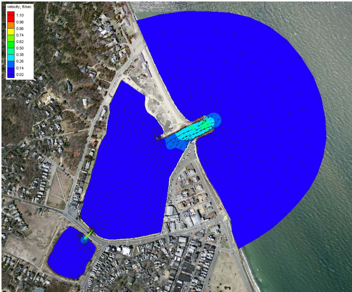
Figure V-14. Example of Oak Bluffs Harbor hydrodynamic model output for a single time step during a spring flood tide at the Oak Bluffs Harbor inlet. Color contours indicate velocity magnitude, and vectors indicate the direction of flow.
