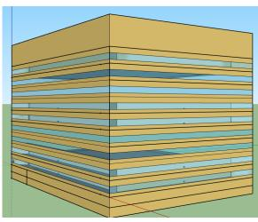
Optimized variations outline both a higher performance, lower capacity Gas-Heating system and an Electric-Heating alternative system along with envelope system improvements. The Office/Lab geometry includes **422,400 gross sf** in nine (9) stories above grade and 2 floor basement levels. Additional 38,357 sf. of penthouse space houses mechanical equipment. The building is slab below grade.
