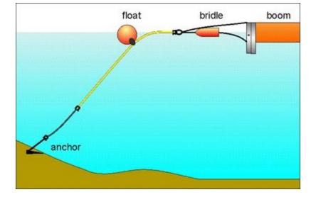
Typical anchor, bridle and boom configuration
