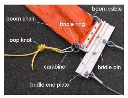
The bridle has a universal end-plate which will attach to all types of booms. It is important to ensure the bridle pin is in place before deployment.
