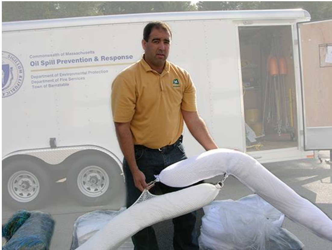
Metal clips link sorbent booms together for adding extra lengths.
