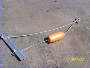
8 Towing Bridles with Thimbles. Is fitted with a universal slide connector to fit both the 18" an 12"
