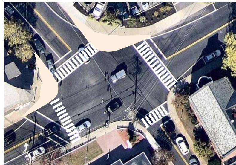
The intersection of Main and North Streets today (above) encourages high speed right turns. Additionally the pedestrian crossings are not designed to be as short as possible. Extending the curbs and painting continental markings (below) will encourage pedestrian safety at a key intersection downtown.
