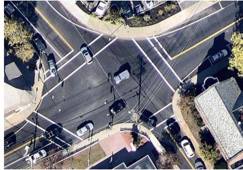
The intersection of Main and North Streets today (above) encourages high speed right turns. Additionally the pedestrian crossings are not designed to be as short as possible. Extending the curbs and painting continental markings (below) will encourage pedestrian safety at a key intersection downtown.
