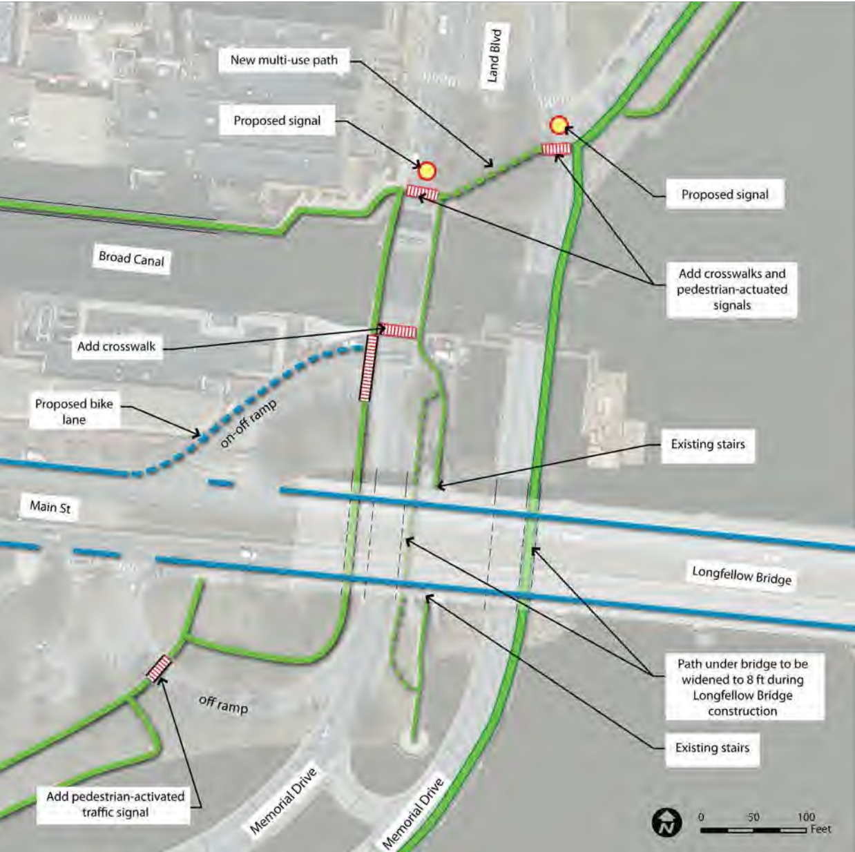
74. Plan diagram showing connectivity improvements where the Broad Canal meets the Charles River
