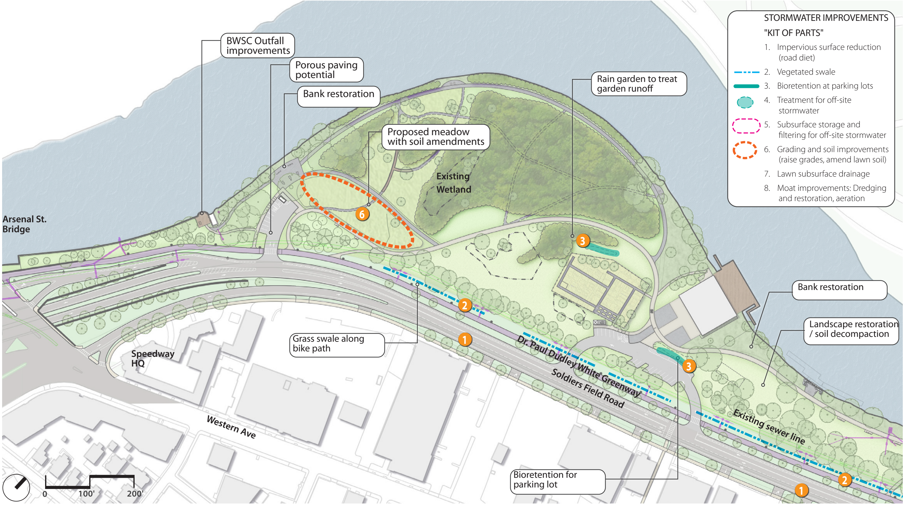
Figure 3-32. West area stormwater improvements.
