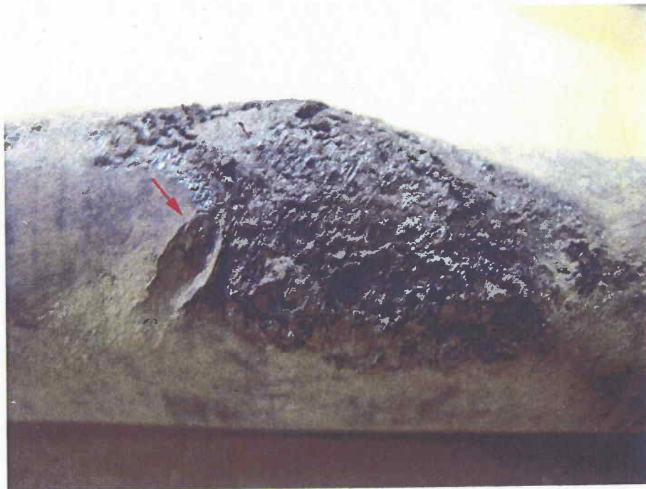
Figure 26: A bubbled region with mark that fits the tracer wire, arrow.
