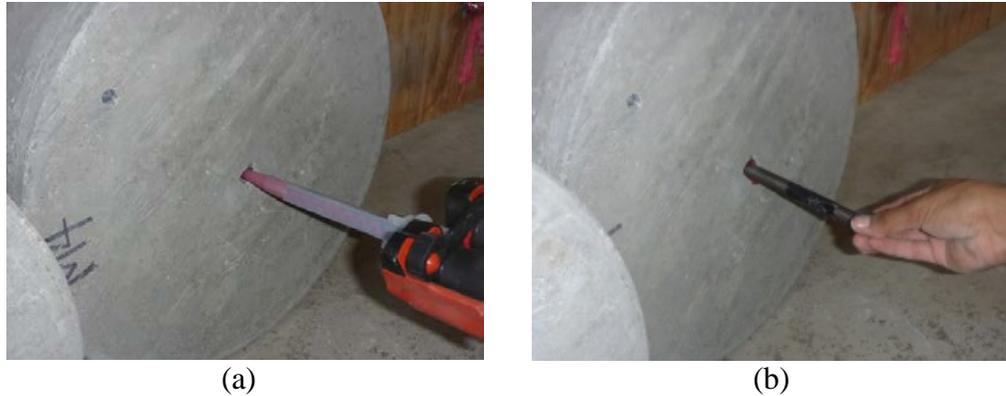
**Figure 4.7: (a) Delivery of adhesive into horizontally drilled hole; (b) horizontal anchor installation**
