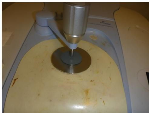
**Figure 6.4: FTIR test of epoxy sample**
