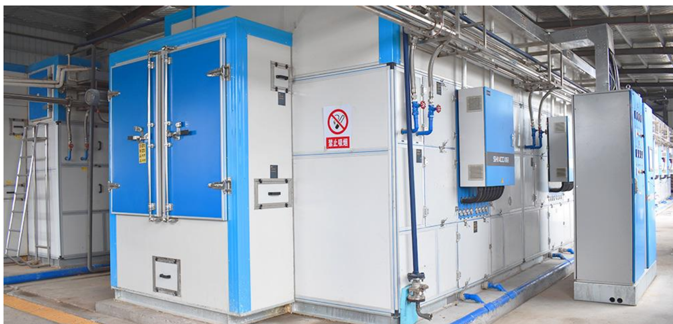
Figure D- 20. Representative Heat Pump Belt Dryer Photograph
