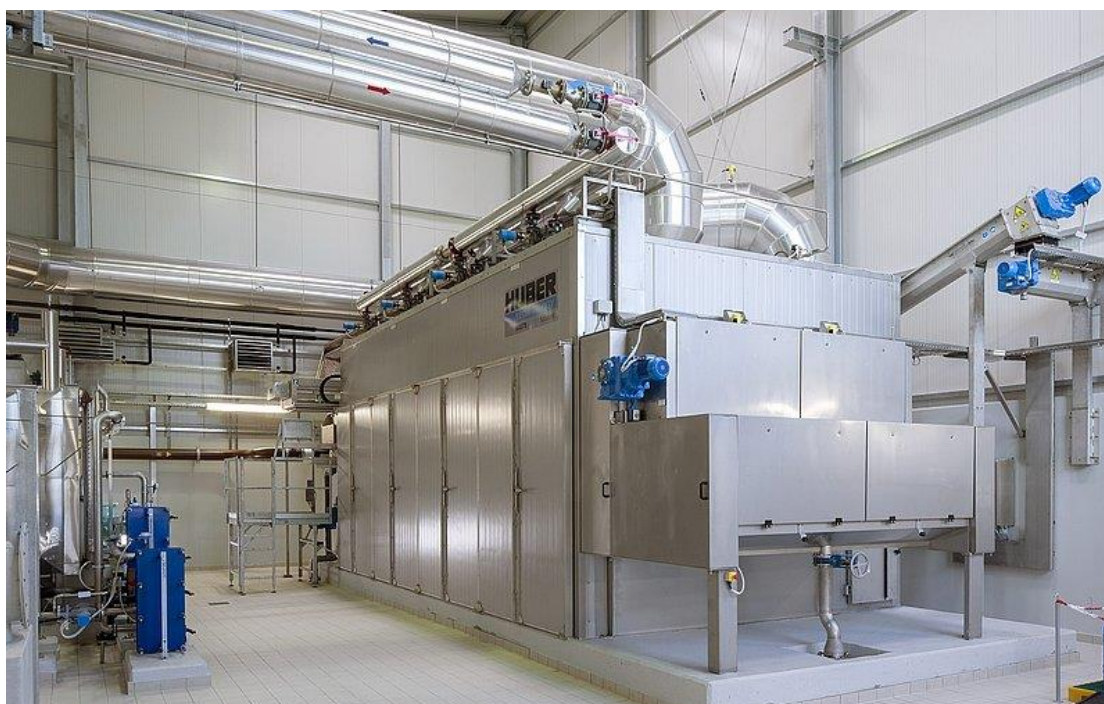
Figure D- 16. Representative Indirect-Fired Belt Dryer Operation Schematic
