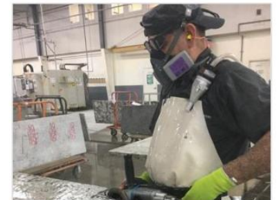
A stone countertop worker uses a grinding tool to alter a countertop.
