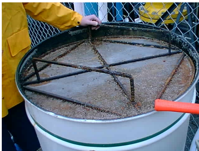
Figure 6: Phase 1 test showing screen on top of PolyGuard Media.
