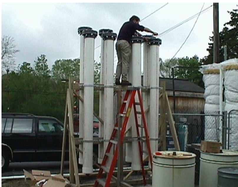
Figure 8: Phase 3 pilot absorption beds shown in mounting rack during construction.
