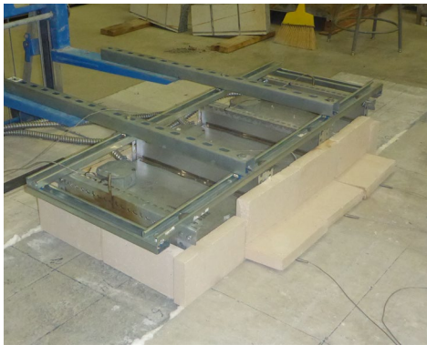
Figure 7.6: Typical Insulation setup. Heating setup before adding any insulation (top); firebrick around heaters (bottom L); insulation around firebrick (bottom R)
