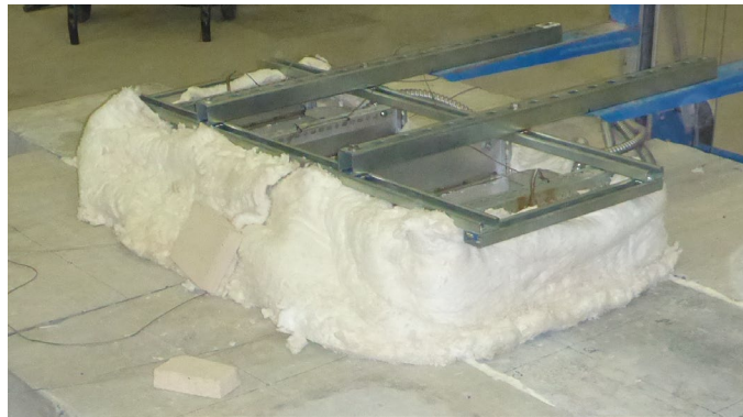
Figure 7.6: Typical Insulation setup. Heating setup before adding any insulation (top); firebrick around heaters (bottom L); insulation around firebrick (bottom R)
