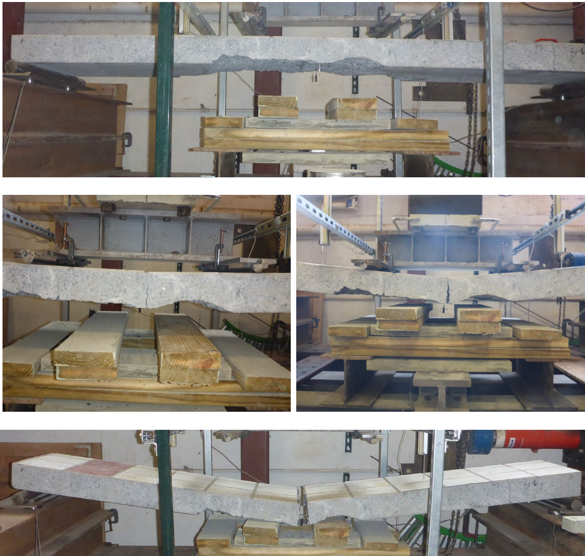
Figure 7.38: Photos of 600°C spalled specimen load testing. Prior to loading (top); propagation of crack during load application (center L and R); after failure (bottom)
