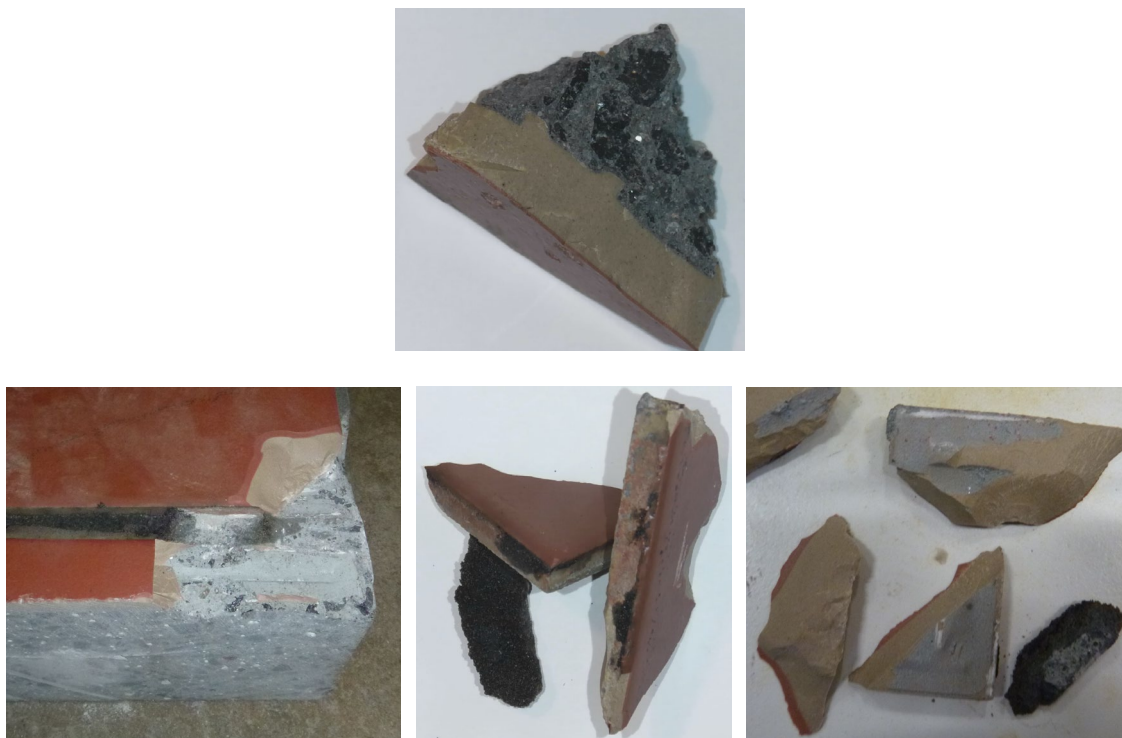
Figure 7.18: Tile and grout removal by chipping hammer and chisel. Unheated specimen (top); specimen heated to 470°C with clean break at grout line (bottom)
