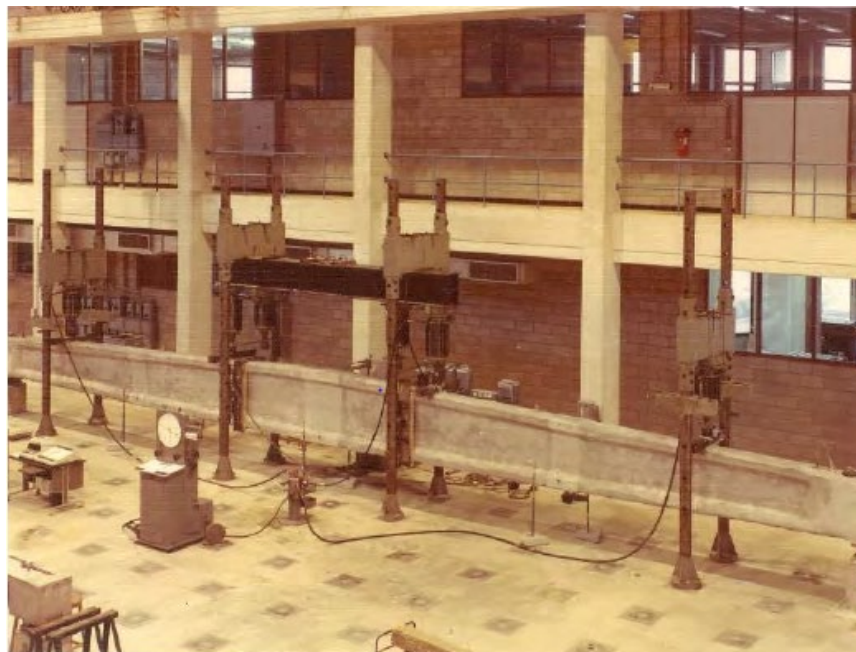
Figure 5.13: Load testing setup for girder
