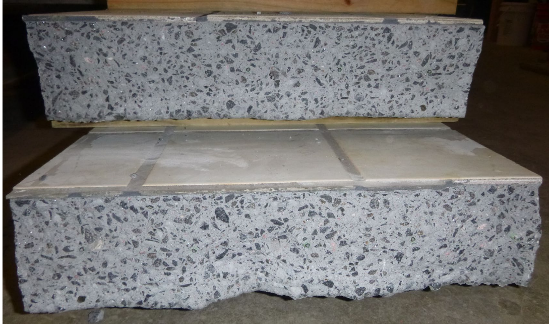
Figure 7.40: Ruptured surface of 300°C heated specimen
