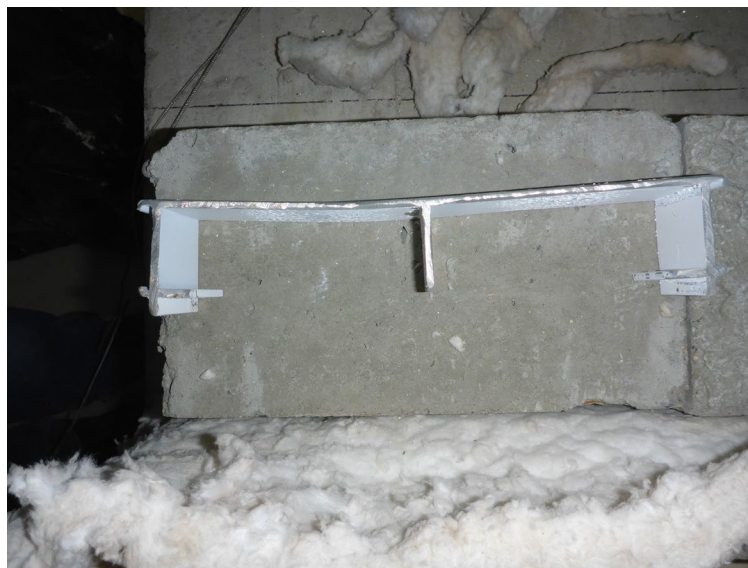
Figure 7.20: Sagging of aluminum wireway after heating
