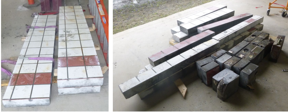
Figure 7.10: Specimens obtained from panel: three primary beams (L), blocks, smaller beams, and miscellaneous (R)
