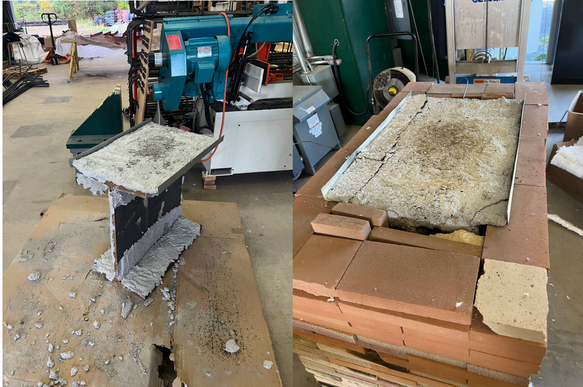
Figure 3-13: Fireproofing on the scenario 3 beam before (left) and after (right) testing
