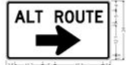
SP-9 1.5" Radius, 0.6" Border, 0.4" Indent, Black on Orange, "ALT ROUTE" - C, 75% spacing, Standard Arrow Custom 18.0" x 12.0" (R)
