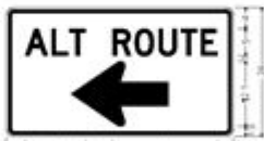
SP-15 1.5" Radius, 0.6" Border, 0.4" Indent, Black on Orange, "ALT ROUTE" - C, 75% spacing, Standard Arrow Custom 18.0" x 12.0" (R)
