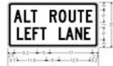
SP-14 1.5" Radius, 0.6" Border, 0.4" Indent, Black on Orange, "ALT ROUTE" - C, "LEFT LANE" - C, 75% spacing
