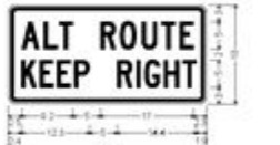
SP-10 1.5" Radius, 0.6" Border, 0.4" Indent, Black on Orange, "ALT ROUTE" - C, "KEEP RIGHT" - C, 75% spacing
