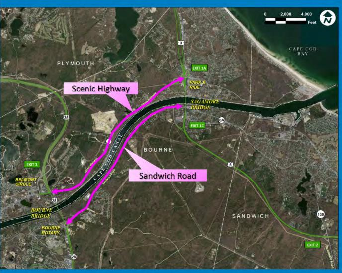
Scenic Highway and Sandwich Road, which parallel the Cape Cod Canal, act as east/west connectors linking the two bridges and are owned by MassDOT.
