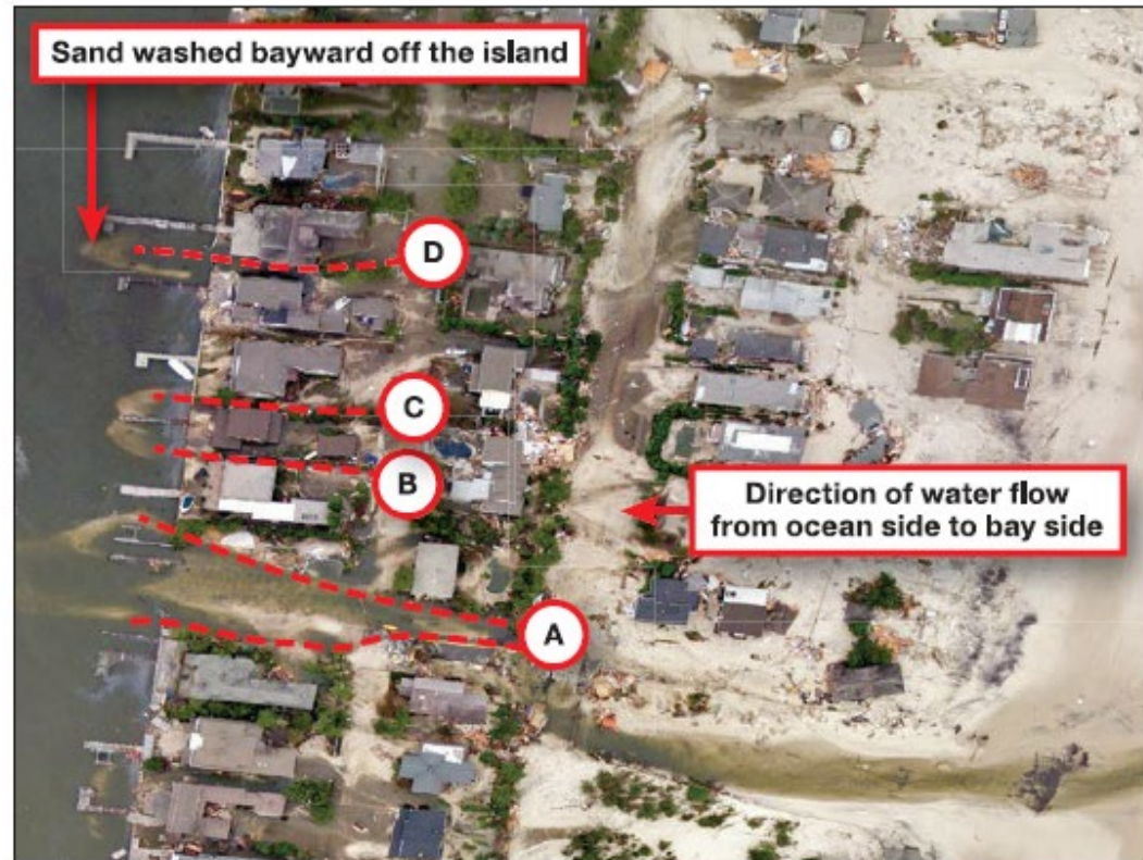
Figure 3-10: Flow channels A–D (dashed lines) formed between buildings on the bayward side of the barrier island at Mantoloking, NJ, and washed sand into the bay at their ends
