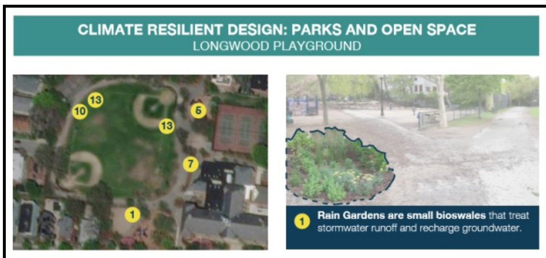
Low-Impact Design recommendations for Longwood Playground in Brookline. Source: Brookline MVP FY18 Action Grant report.
