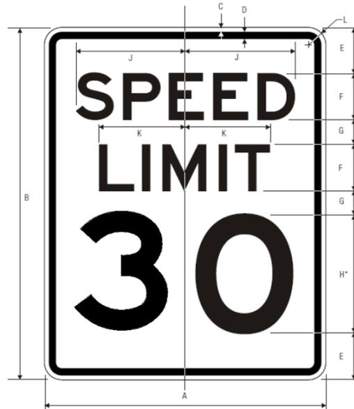
**Fig. 9-1: Standard R2-1 (Speed Limit) Sign with Dimensions**
