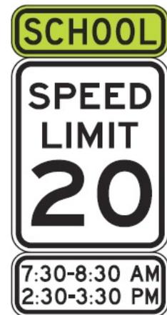
Fig. 10-4: R2-1 Sign with S4-3P and S4-1P Plaques (Source: MUTCD)
