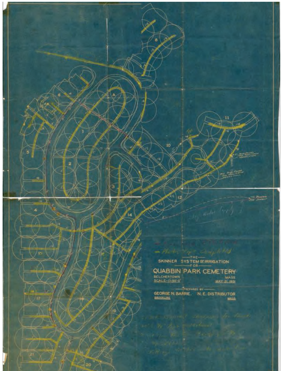
Figure 4-33. Layout of the original irrigation system.
