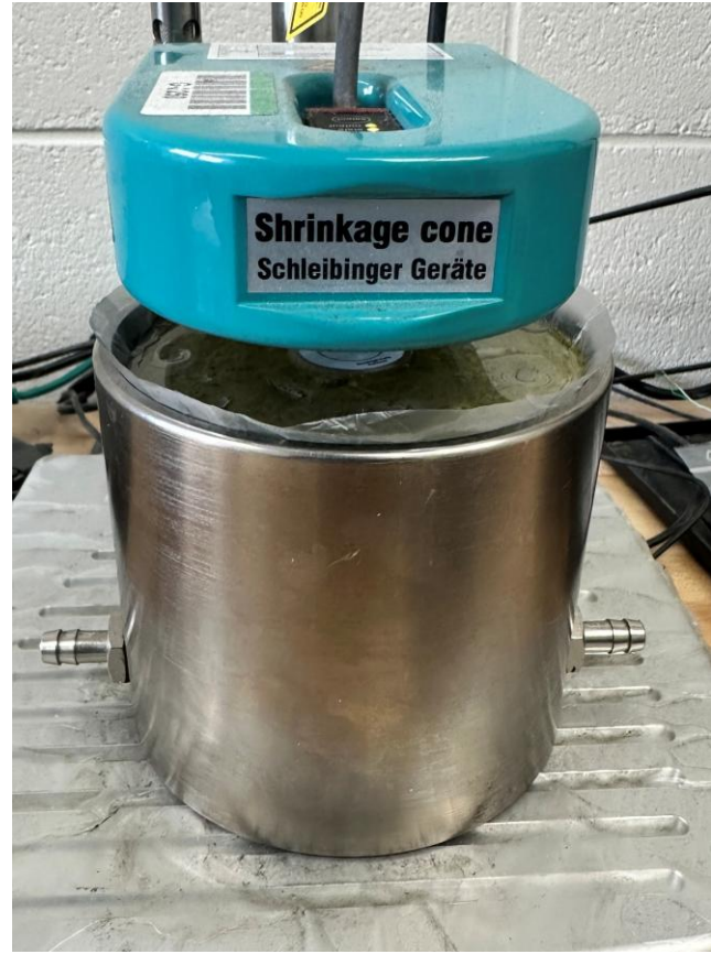
Figure 3.9: Laser-based shrinkage cone for early-age shrinkage measurement.
