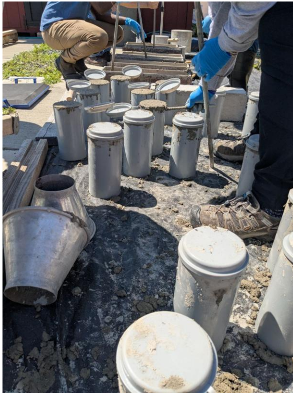
Figure 3.15: 4 by 8-inch cylinder mold filling process
