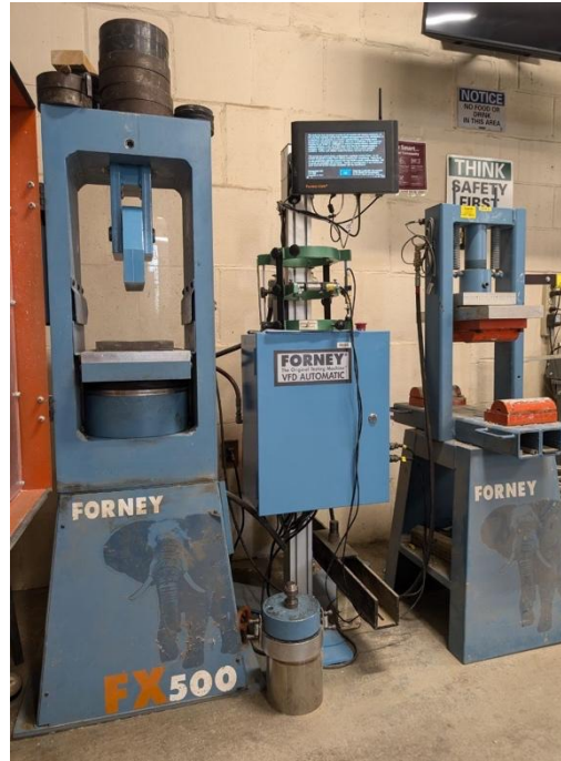
Figure 3.10: Forney testing machine used for compression, splitting tensile tests, and four-point bending tests
