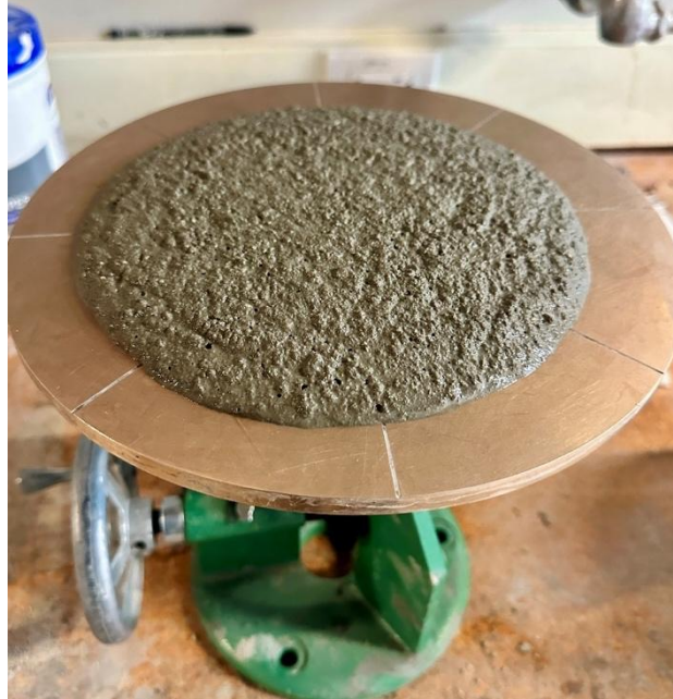
Figure 3.8: Flowability test of RGGP-modified mortar
