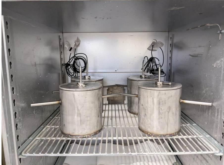
Figure 3.28: Fully assembled ACCT test setup inside an oven
