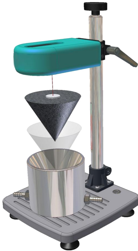
Figure 3.9: Laser-based shrinkage cone for early-age shrinkage measurement.
